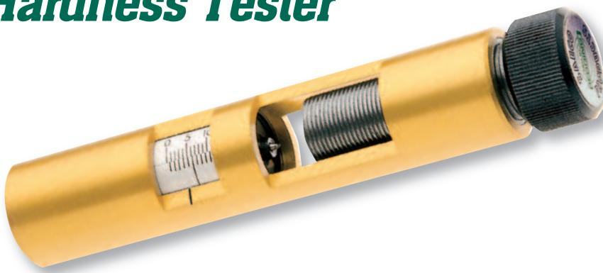
A SAEKO Lead Hardness Tester will pay for itself many times over by allowing you to convert inexpensive scrap lead of unknown composition into casting alloy of known and reproducible hardness. It provides a standard by which you can check the quality of purchased cast bullets. The SAEKO Lead Hardness Tester measures alloy hardness by determining the depth of penetration of a hardened steel indenter into a bullet. Relative hardness of the bullet is read off a vernier scale.
