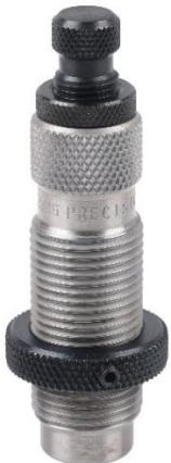
Precision Expanding Dies are machined on CNC Lathes and heat-treated to ensure dimensional integrity and durability for a lifetime of use. The unique angled alignment surfaces of the Die Body and Mandrel ensure perfect alignment when assembled and secured with the threaded retention plug and lock ring.
