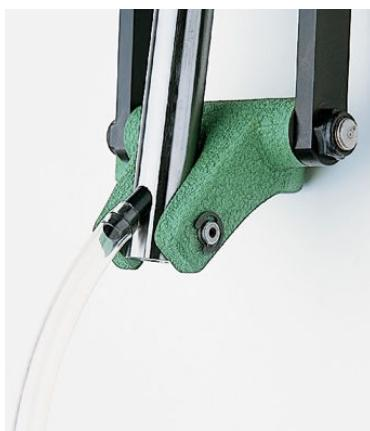
The unique spent primer collection system on the Big Boss II reloading press routes the spent primer and its associate debris through the ram and into a collection tube on the rear of the ram at its base. The tube can retain hundreds of primers and is emptied by removing the knurled metal plug at its end. This system keeps the top of the press and the surrounding work area clean and free of debris.
