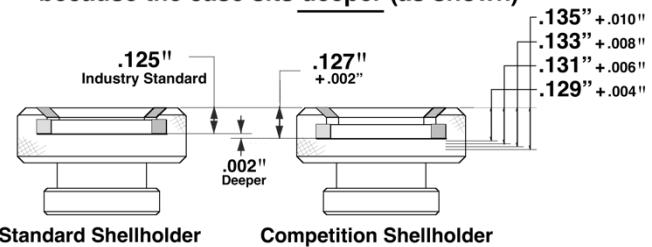
the empty cartridge case does not chamber or chambers with difficulty, switch to the shellholder marked +.008 and repeat the process. Do not readjust the die.
